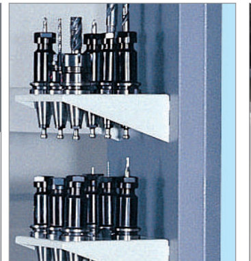
Convenient & easy to use tool stand including tool-locked device.
