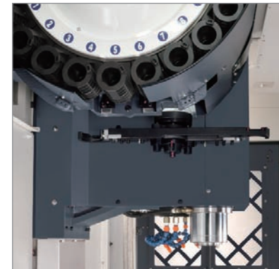
Arm type tools: The fast, simple and long-life automatic tool changer provide stable and reliable toolchange.
