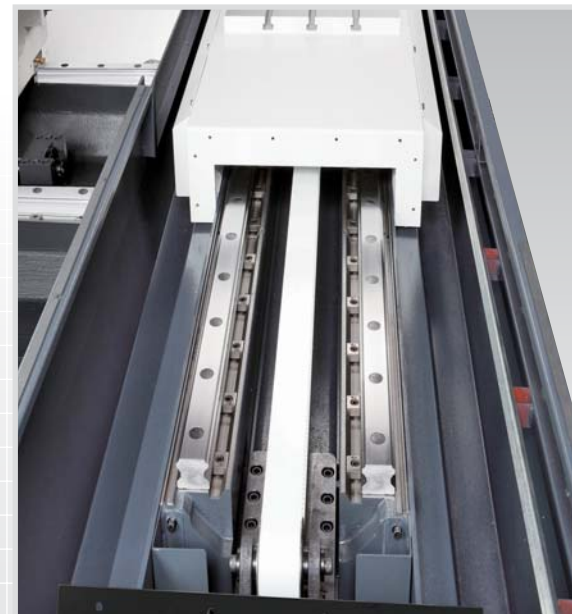
X axis direct drive transmission mechanism, collocated with super precision Roller type guide way. (Belt drive is available as option.)
