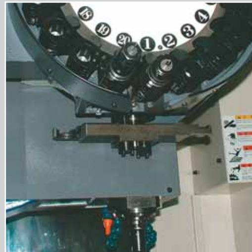
Arm type ATC 20 tools: The fast, simple and long-life automatic tool changer provide stable and reliable tool change.
