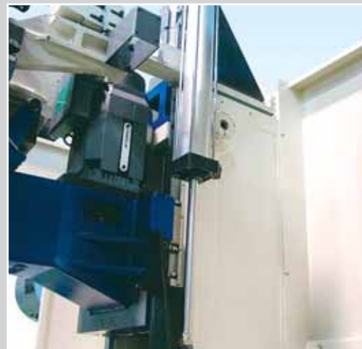
Air pressure counterweight mechanism to uplift for Z axis screw and motor.
