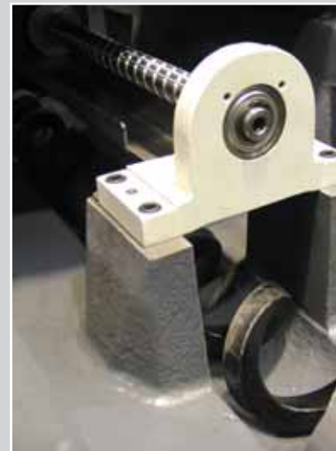
A simple but efficient removal mechanism can easily move the chips to rear side of the machine.
