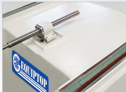
Enlarge double V base. These guide ways are equipped with auto lubrication to resist wear of guide ways, plus lasting accuracy & damping.
